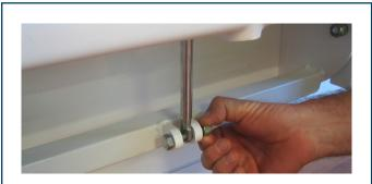
**Gas Strut Check** Ensure gas strut is secure, tight and functioning properly.
