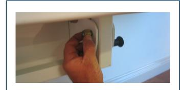
**Bed Base Check** Check the bed base hinge bolts are secure and tight.
