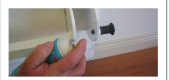
**Moving Parts Check** Spray moving parts and locks with some lubricant spray – this will enhance longer life to wearing parts.
