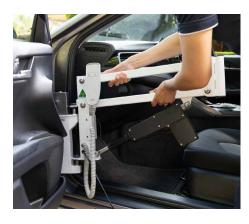
The frame of the IBIS is placed and Once this is secure, place the secured over the two lugs in the bracket.
