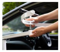
Connect the chest bar into the extension bar. Ensure the hoist is secure.
