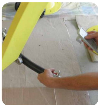
2. Lower arm until lifting hanger just touches the ground.
