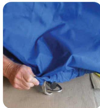
4. Pull cover over lifting hanger.
